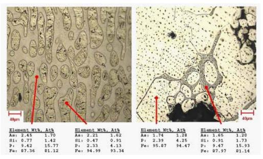
Fig. 4. Metallographic picture of iron bloom samples (200x). a. iron bloom made of Fancsika iron ore b. iron bloom made of Petesmalom iron ore.
