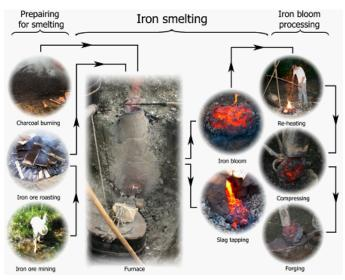
Fig. 2. The steps of the early medieval iron manufacturing.
